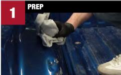
Pressure wash and allow to dry. Clean with **SEM Solve** or **XXX Universal Surface Cleaner**. Wipe clean in one direction with dry, lint-free cloth.
