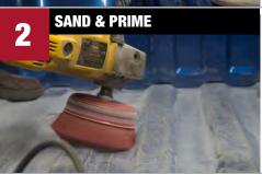
Remove all rust. Sand inside of bed with P180 – P220 grit or a bed brush. Truckbed liners may be sprayed over OEM finishes.
